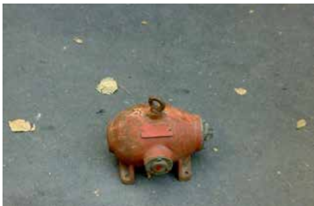
■ A typical container for highly-radioactive Cesium-137, referred to as “piglet” in smugglers’ jargon (Credit: State Security Service of Georgia).
